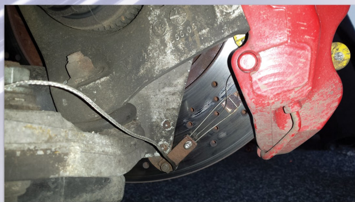
Above, rubbing thermocouple installation
